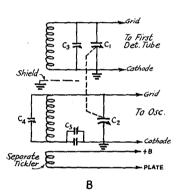
FIG. 617 — CONVERTER CIRCUIT TRACKING METHODS
