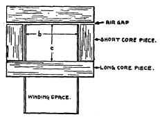
FIG. 1525 — CORE ARRANGEMENT FOR FILTER CHOKE COILS
