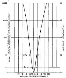
FIG. 602—A TYPICAL RECEIVER SELECTIVITY CURVE OBTAINED BY PLOTTING MICROVOLTS INPUT, AT VARIOUS INTERMEDIATE FREQUENCIES, REQUIRED TO GIVE CONSTANT AUDIO OUTPUT. THE TEST SIGNAL IS OBTAINED FROM A STANDARD SIGNAL GENERATOR
