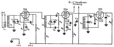
FIG. 1318 — WIRING OF THE ACORN INPUT UNIT  $L_1$ —Seven turns of No. 15 enamelled wire ½-inch inside
