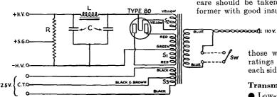
FIG. 1511 — WIRING DIAGRAM OF THE POWER SUPPLY SHOWN IN FIG. 1510
