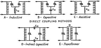
FIG. 407 -- BASIC TYPES OF CIRCUIT COUPLING
