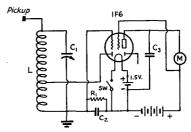
FIG. 1721 — THE TWO-STAGE FIELD-STRENGTH METER CIRCUIT DIAGRAM
