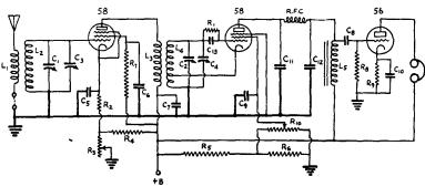
FIG. 713-A — CIRCUIT DIAGRAM OF THE "OLD RELIABLE" RECEIVER
