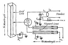
FIG. 1418—ILLUSTRATING THE USE OF CON-CENTRIC LINES IN THE FILAMENT CIRCUIT OF A TRANSMITTER FOR THE ULTRA-HIGH FREQUENCIES
