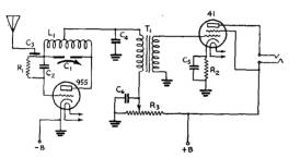
FIG. 1306 — CIRCUIT OF THE "ACORN" RECEIVER
