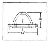
H.F. BUSHING. A heavy bowl-type lead-in, suitable for large transmitters, this Steatite insulator provides a weatherproof joint for antenna lead-in purposes. Leakage Path 31/4".
