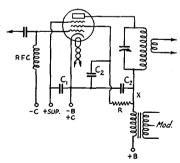
FIG. 1212 — PENTODE PLATE-MODULATION CIRCUIT WITH SCREEN-DROP RESISTOR
