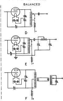
FIG. 1613 — COUPLING THE SINGLE WIRE Untuned transmission line to balanced and unbalanced output circuits.
