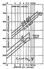
FIG. 1618 — GRAPHICAL TABLE OF CHARACTER-ISTIC IMPEDANCES OF TYPICAL SPACED-CON-DUCTOR TRANSMISSION LINES
