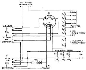
FIG. 1712 — COMBINATION MULTI-RANGE OHM-METER, MILLIAMMETER AND A.C.-D.C. VOLTMETER
