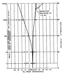
FIG. 622 — MAXIMUM CRYSTAL SELECTIVITY CURVE FOR THE FILTER CIRCUIT OF FIG. 621-A
