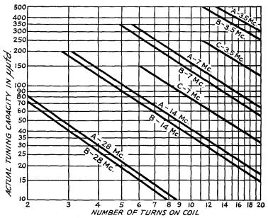
FIG. 832 — WINDING DATA FOR COPPER-TUBING
