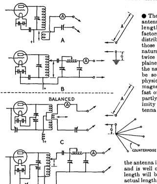
FIG. 1602 — THE MARCONI ANTENNA WITH VARI-OUS METHODS OF COUPLING
