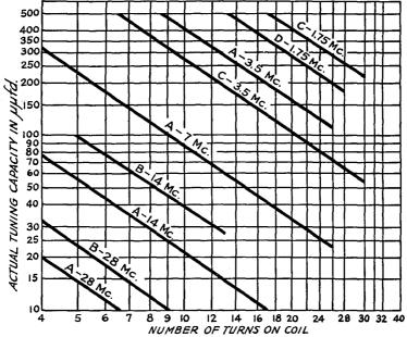
FIG. 831 — COIL-WINDING DATA FOR CERAMIC TRANSMITTING-TYPE FORMS
