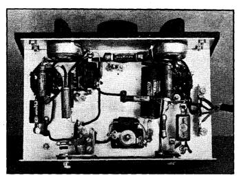
FIG. 1311 — THE UNDERSIDE OF THE METAL-TUBE RECEIVER Plate and screen by-pass condensers for the detector are run directly to one point on the chassis immediately under the tuning condenser mounting. All other leads are made short and direct chiefly to give greater rigidity.
