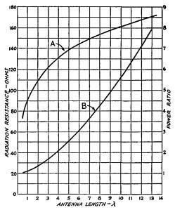
FIG. 1603 — THE IMPORTANT CURVES FOR HAR-MONICALLY-OPERATED HORIZONTAL ANTENNAS
