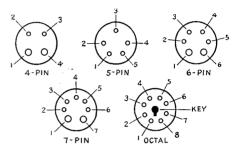
FIG. 516 — TUBE-BASE PIN NUMBERING SYSTEM
