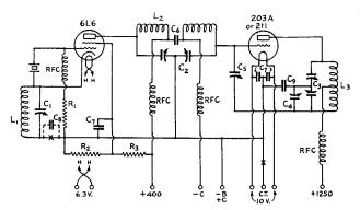
FIG. 935 - CIRCUIT DIAGRAM OF THE 100-WATT TRANSMITTER
