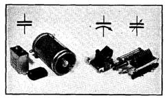
FIG. 304 — TYPES OF FIXED CONDENSERS (LEFT) AND VARIABLE CONDENSERS (RIGHT) WHICH ARE USED IN RADIO CIRCUITS
