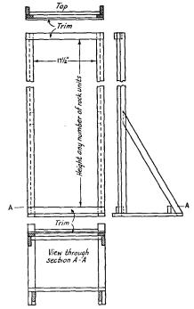
FIG. 903 — SUGGESTED CONSTRUCTION OF AN INEXPENSIVE WOODEN RELAY RACK
