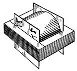
FIG. 1524 — A CONVENIENT METHOD OF ASSEMBLING THE WINDINGS ON A SHELL TYPE CORE
