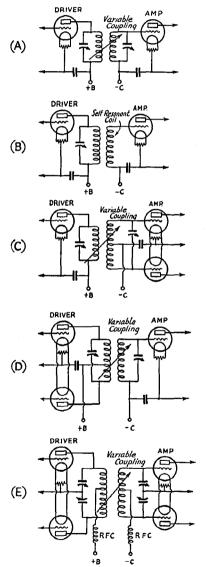
FIG. 815 - INDUCTIVE INTERSTAGE COUPLING
