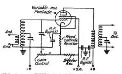
FIG. 605 — A TYPICAL RADIO-FREQUENCY AMPLIFIER CIRCUIT WITH BIAS GAIN CONTROL
