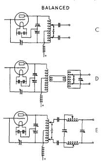
FIG. 1624 — SUITABLE METHODS FOR COUPLING OUTPUT CIRCUITS TO ALL TYPES OF TWO-WIRE UNTUNED TRANSMISSION LINES INCLUDING TWISTED PAIR LINES, CONCENTRIC LINES AND OPEN WIRE LINES
