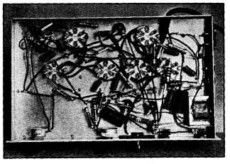
FIG. 721—A BOTTOM VIEW OF THE SIX-TUBE SUPERHET By-pass condensers and resistors are placed in the most convenient locations. The detector output transformer is mounted on the side wall of the chassis, and can be seen in the lower right-hand
