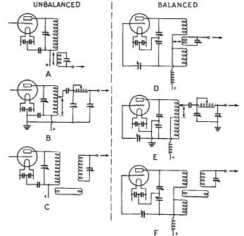
FIG. 1606 — SEVERAL SUGGESTIONS FOR COUPLING THE END OF VOLTAGE-FED ANTENNA
