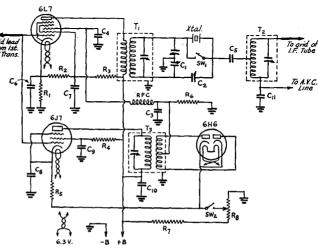
FIG. 728 — CIRCUIT DIAGRAM OF THE CRYSTAL FILTER AND NOISE-SILENCER UNIT
