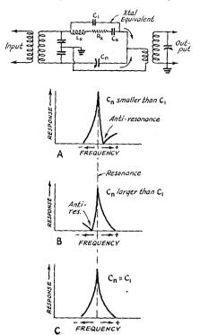
FIG. 624 — THE REJECTION ACTION OF THE S.S. CRYSTAL FILTER CIRCUIT
