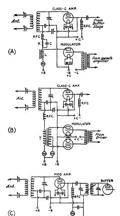
FIG. 1103 — CIRCUITS FOR THREE METHODS OF MODULATION
