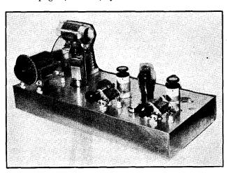
FIG. 924 — A THREE-BAND TWO-STAGE PENTODE TRANSMITTER A 59, pentode or Tri-tet, drives an RK-20 or 804 amplifier, using 3.5-and 7-mc, crystals. No buffer stages are needed. This outfit was built by W1AF,
