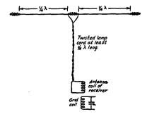
FIG. 1630 - DOUBLET RECEIVING ANTENNA
