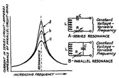
FIG. 402 — CHARACTERISTICS OF SERIES-RES-ONANT AND PARALLEL-RESONANT CIRCUITS
