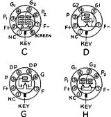
nection be grounded, however, to provide for possible metal-shell tubes in this series. (Note: In some cases the tube may be provided with more pins than are indicated in the above diagrams. This is a manufacturing convenience; the extra pins have no connections and can be ignored.)
