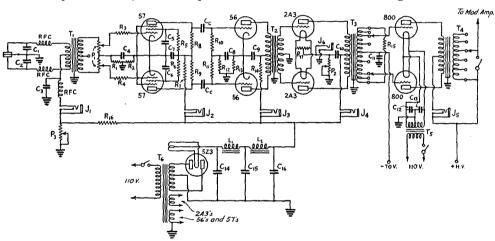
FIG. 1209 — CIRCUIT OF THE 100-WATT AUDIO SECTION
