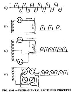
At (1) is the conventional representation of the a.c. vave; (2) shows a half-wave rectifier; at (3) is the full-wave center-tap system; and (4) is the "bridge" rectifier. The output wave form with each type of rectifier is shown at the right.
