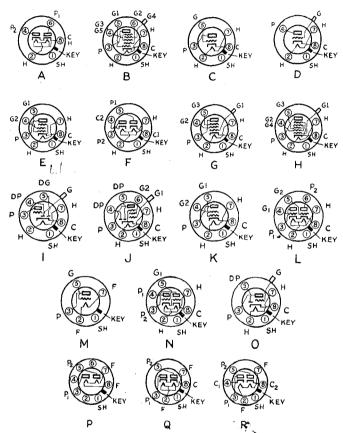
FIG. 518 — BASE DIAGRAMS OF METAL AND 6.3-VOLT "G" TYPE RECEIVING TUBES É
