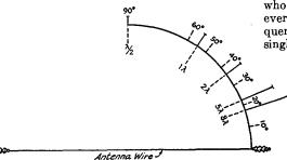
FIG. 1629 — ANGLES OF MAXIMUM RADIATION, MEASURED FROM THE LINE OF THE ANTENNA, FOR ANTENNAS OF DIFFERENT LENGTHS IN TERMS OF THE OPERATING WAVELENGTH
