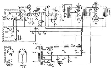
FIG. 1203 — CIRCUIT OF THE GENERAL-PURPOSE 18-WATT AUDIO UNIT
