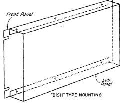
902 - THE "DISH" TYPE OF SUB-PANEL MOUNTING FOR THE RELAY RACK
