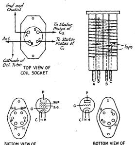
FIG. 708—TUBE AND COIL SOCKET CONNECTIONS, SHOWING THE METHOD OF WINDING THE COILS ACCORDING TO THE FOLLOWING SPECIFICATIONS
