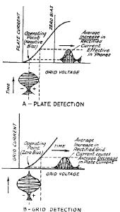
FIG. 513 — OPERATING CHARACTERISTICS OF PLATE AND GRID DETECTORS
