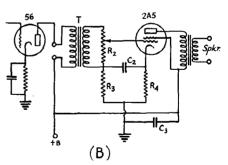
FIG. 711 - CIRCUITS OF POWER AMPLIFIERS FOR TWO-TUBE RECEIVERS, THAT OF B BEING PREFERRED
