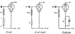
FIG. 824 — AMPLIFIER BIASING METHODS
