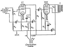
FIG. 1202 - CIRCUIT OF A SIMPLE SPEECH-AM-PLIFIER AND MODULATOR SUITABLE FOR LOW-POWER PLATE MODULATION, OR FOR SUPPRES-SOR- OR CONTROL-GRID MODULATION
