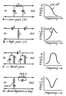
FIG. 410 — TYPES OF FILTERS AND APPROXIMATE CHARACTERISTICS OF EACH
