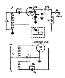
FIG. 1308 — TWO TYPICAL METHODS OF APPLY-ING QUENCH VOLTAGE TO THE SUPERREGENER-ATIVE DETECTOR
