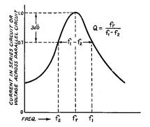
FIG. 403 — HOW THE VALUE OF Q IS DETERMINED FROM THE RESONANCE CURVE OF A SINGLE CIRCUIT
