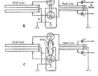
a quarter wave — it would be exactly a quarter wave if it were not for the loading offered by the capacity of the vacuum-tube elements.
