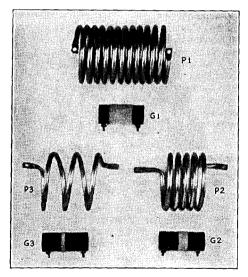
FIG. 802 — TYPICAL HIGH-C COILS FOR THE SELF-CONTROLLED OSCILLATOR
