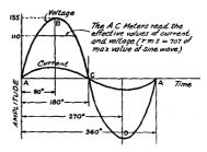
FIG. 306 — REPRESENTING SINE-WAVE ALTER-NATING VOLTAGE AND CURRENT
