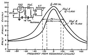
FIG. 406 — RESONANCE CURVES OF TWO PRACTICAL CRYS-TAL RESONATORS, SHOWING THEIR HIGH O
