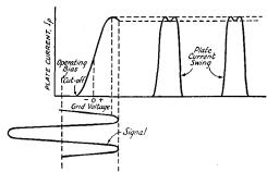
FIG. 510 - CLASS-C AMPLIFIER OPERATION
