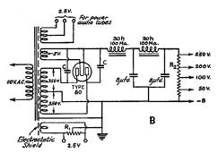
FIG. 1516 — WIRING DIAGRAMS FOR RECEIVER POWER SUPPLIES
