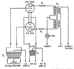
FIG. 1211 — CIRCUIT OF THE 500-WATT CLASS-B MODULATOR
