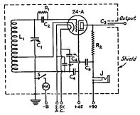
FIG. 1705 — CIRCUIT OF THE ELECTRON-COUPLED FREQUENCY METER
