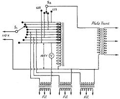
FIG. 1522 — WITH THIS CIRCUIT, A SINGLE ADJUSTMENT OF SWITCH S<sub>1</sub> PLACES THE CORRECT PRIMARY VOLTAGE ON ALL TRANSFORMERS IN THE TRANSMITTER
