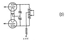
FIG. 825—METHODS OF SWITCHING THE AM-PLIFIER PLATE TANK CIRCUIT FOR CHANGING BANDS
