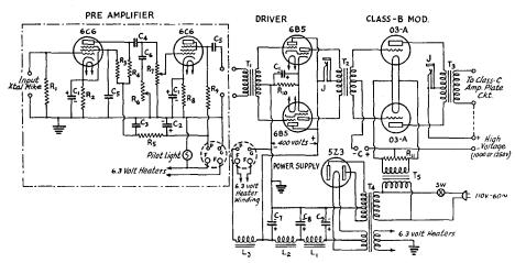
FIG. 1210 — COMPLETE CIRCUIT OF THE 250-WATT DRIVER-MODULATOR AND PRE-AMPLIFIER UNITS
