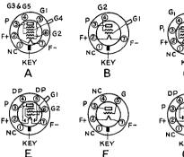
FIG. 518-A — SOCKET-CONNECTION DIAGRAMS FOR OCTAL-BASED 2.0-VOLT TUBES
