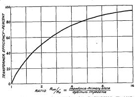
FIG. 813 — VARIATION OF COUPLING TRANS-FORMER EFFICIENCY WITH TUNED CIRCUIT IMPEDANCE
