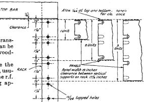
FIG. 901 - DRILLING AND PANEL DIMENSIONS OF THE STANDARD RELAY RACK
