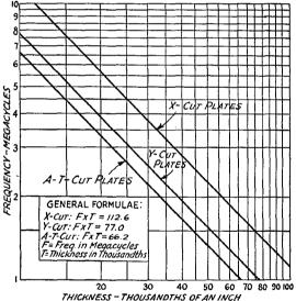
OF X-, Y- AND AT-CUT PLATES
