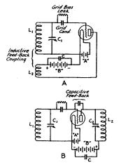
FIG. 511 — TWO GENERAL TYPES OF OSCILLATOR CIRCUITS
