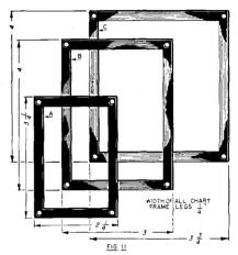
COIL CHART FRAMES: Nickel Silver Chart Frames are available in the sizes shown above. The largest frame is the same as that used on the AGS, the medium frame is the same size as that on the FB-7, and the smallest is the same as the HRO frame. Prices include celluloid sheet to protect the chart.
