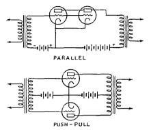
FIG. 506 — PARALLEL AND PUSH-PULL AMPLIFIER CONNECTIONS
