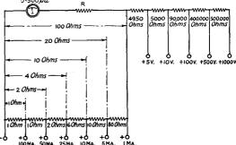
FIG. 1711 - A MULTI-RANGE VOLTMETER-MILLIAM-METER USING A 0-500 MICROAMMETER
