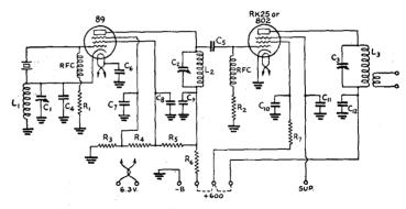
FIG. 917 — CIRCUIT DIAGRAM OF THE TWO-STAGE EXCITER UNIT
