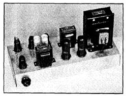
FIG. 1204 — METAL-TUBE SPEECH UNIT WITH PUSH-PULL 6L6 OUTPUT
