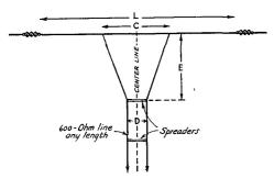
FIG. 1615 — TWO-WIRE MATCHED-IMPEDANCE ANTENNA SYSTEM
