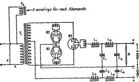
FIG. 1512 - A DUPLEX PLATE SUPPLY CIRCUIT
