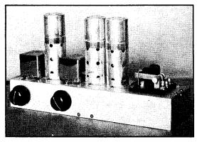
VOICE-OPERATED RELAY FOR 'PHONE OPERATION This electronic relay utilizes the circuit described in Fig. 1803. Rather complete shielding is recommended as the gasfilled 885 control tube may cause disturbance in the receiver. Shielded transformers are used.
