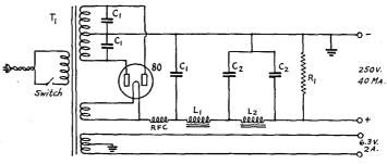
FIG. 1518—A LOW-CURRENT POWER SUPPLY FOR REGENERATIVE OR T.R.F. RECEIVERS
