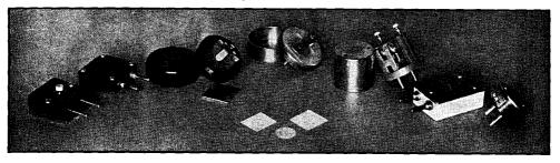
FIG. 806 - CRYSTALS AND CRYSTAL HOLDERS
