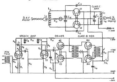
as the one shown in FIG. 1214 -- CLASS-B CONTROLLED-CARRIER CIRCUIT FOR 500-VOLT TYPE TUBES (W2CTK)
