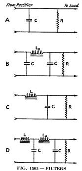
At A is the simplest type of filter—a single condenser of high capacity connected across the rectifier output. With the addition of a filter choke and a second condenser this becomes the "brute force" circuit of B. C is a single-section choke-input filter. The twosection filter at D is recommended when the ripple voltage in the output must be low.
