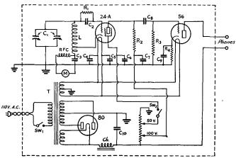
FIG. 1708 - CIRCUIT DIAGRAM OF THE A.C.-OPERATED FREQUENCY METER
