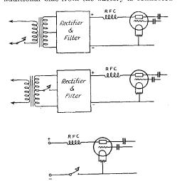
FIG. 1001 — PLATE-KEYING METHODS
