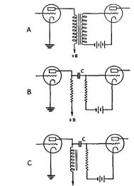
FIG. 507 — METHODS OF COUPLING BETWEEN AMPLIFIER TUBES
