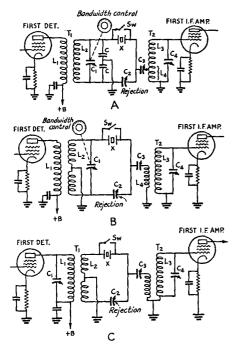
FIG. 621 — THREE TYPES OF CRYSTAL FILTER CIRCUITS
