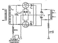
FIG. 1219 — GRID CIRCUIT CHANGES IN THE FINAL AMPLIFIER OF THE GENERAL-PURPOSE TRANSMITTER TO FIT IT FOR GRID-BIAS MODULATION
