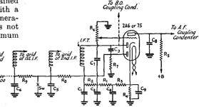
FIG. 626 — THE SECOND DETECTOR-A.G.C.-FIRST AUDIO CIRCUIT
