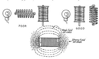
FIG. 906 — THE RIGHT AND WRONG WAY TO MOUNT COILS IN THE
