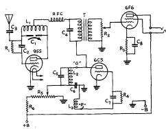
FIG. 1313 — WIRING OF THE ACORN-TUBE RECEIVER
