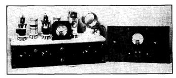
FIG. 927 — A GENERAL VIEW OF THE 50-WATT TRANSMITTER AND THE ANTENNA TUNING UNIT
