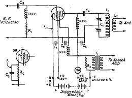
FIG. 1104 — CIRCUIT OF THE SUPPRESSOR-GRID MODULATED R.F. AMPLIFIER
